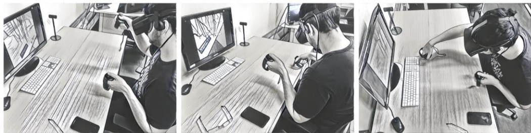
Figure 1. In VirtualDesk, interaction is a combination of mid-air natural gestures and tangible contact with the real-world work desk. Viewpoint changes are only possible by manipulating the dataset or through head movements, greatly reducing simulator sickness.
